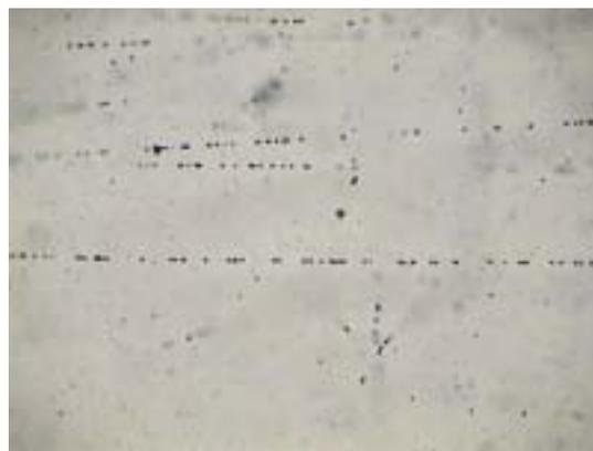
Fig. 1 A recorded trajectory of electron tracks. Horizontal scale is 120 microns.
