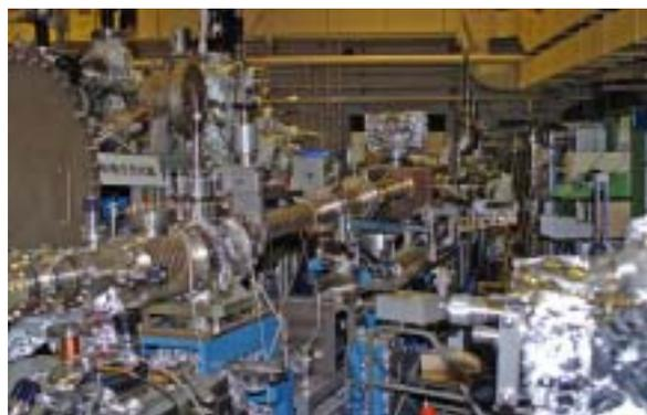
Fig. 1 Photo of the monochromator at BL8B1.
